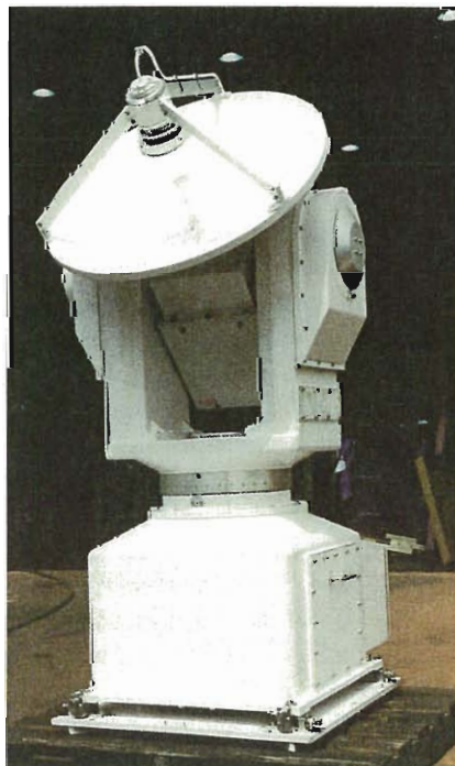
Photo 2. A close-up of an element antenna.
