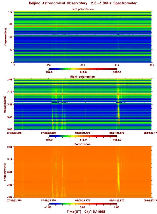
Fig. 4.. The LC, RC, and polarization images of multiple channels with 0.2 s time resolution for the same event.
